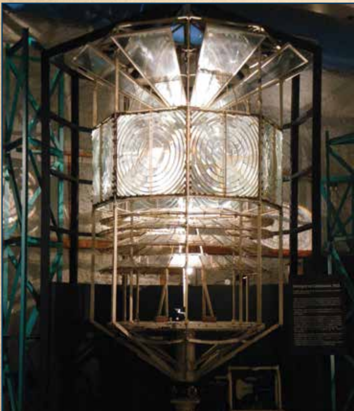
Augustin Fresnel's first lens featured flat rather than curved panels. Note the flat panels mounted at an angle at the top of the lens.
