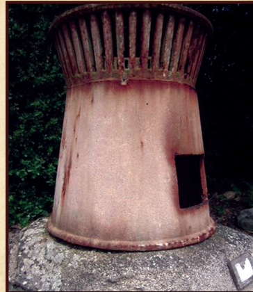
This coal fired cresset (or brazier) was once housed in an open air lantern room perched atop the St. Agnes Lighthouse in Great Britain.
