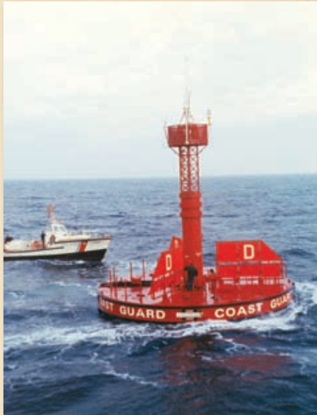
MEASURING 40 FEET HIGH AND 40 FEET WIDE, A LARGE NAVIGATIONAL BUOY (LNB) CAN PASS MANY FEATURES INCLUDING A LIGHT, FOG HORN, RADAR REFLECTOR, AND WEATHER MONITORING EQUIPMENT.
