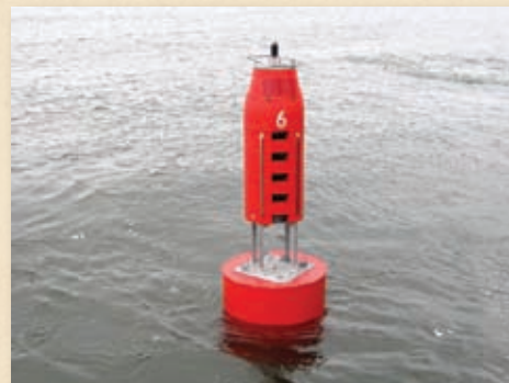
THE COAST IS PHASING OUT ITS OLD STEEL BUOYS AND REPLACING THEM WITH FOAM BUOYS LIKE THE ONE DIAGRAMMED ABOVE AND PICTURED BELOW.
