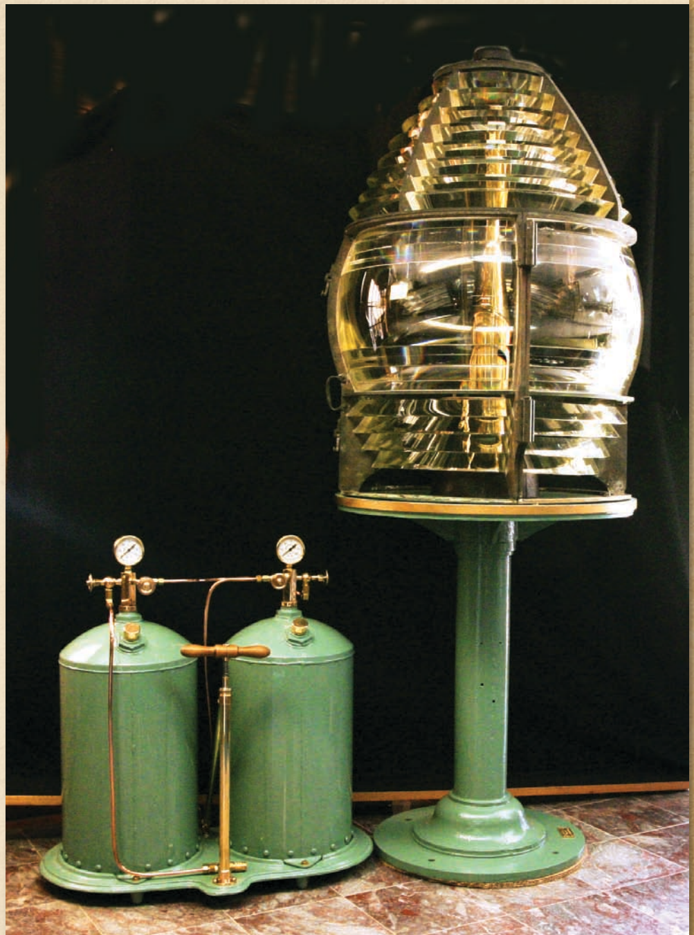
CHANCE BROTHERS LENS WITH PEDESTAL, FUEL TANKS, AND INCANDESCENT OIL VAPOR LAMP.
