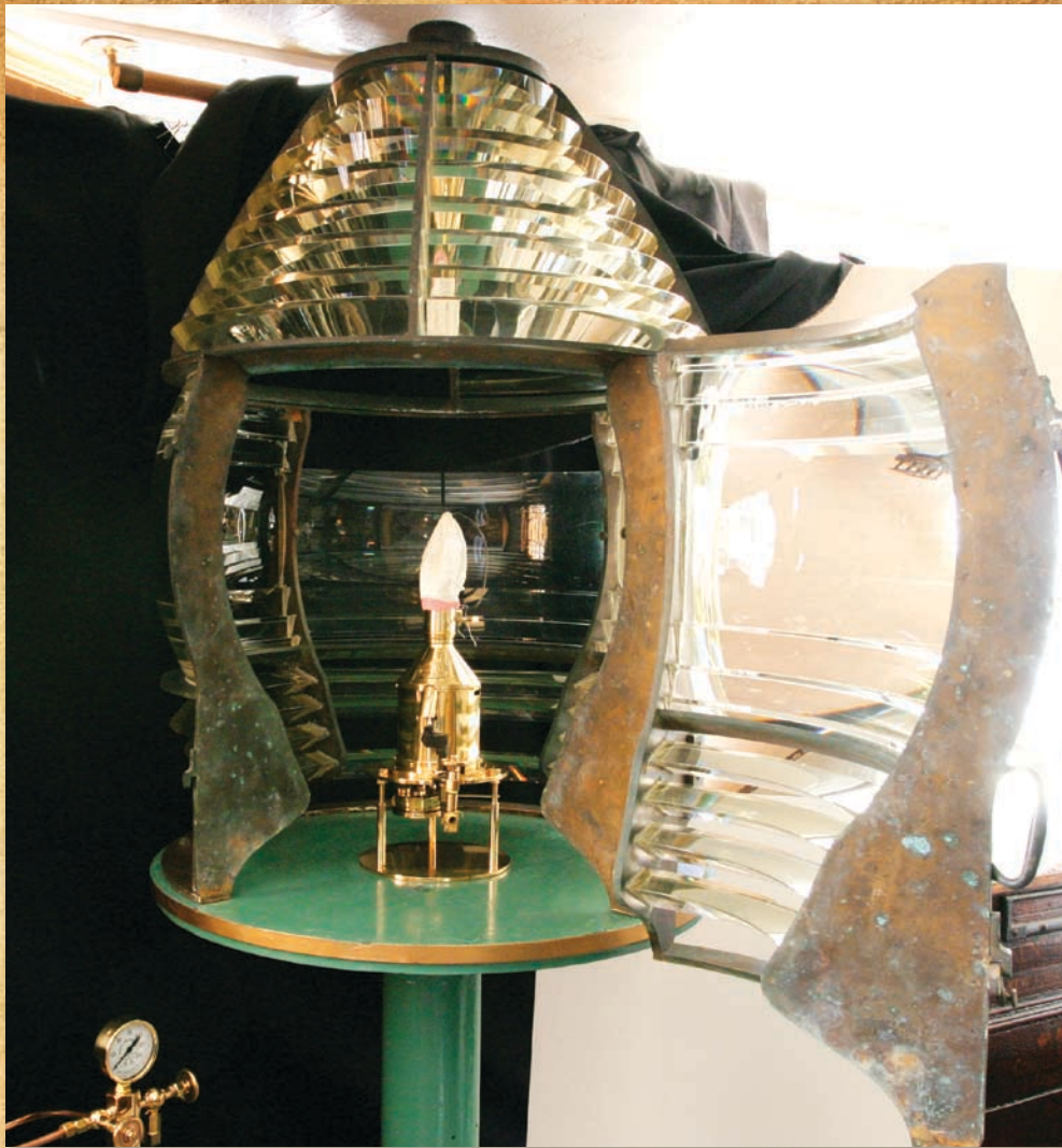
CHANCE BROTHERS LENS WITH DOOR OPEN TO REVEAL INCANDESCENT OIL VAPOR LAMP.
